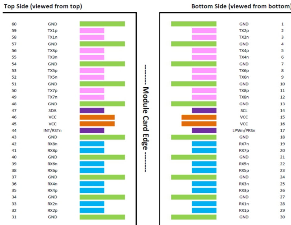
Figure 6: OSFP Module Pinout
